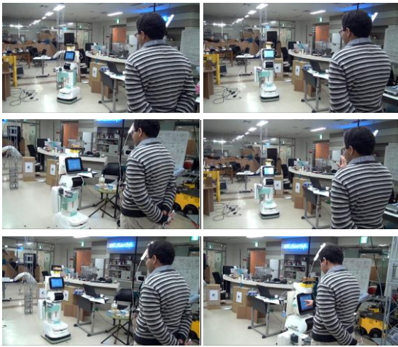
Figure 18. Calling gesture recognition in robot system test. The picture above are the screen shots of calling gesture demo, [27] show the full demo
